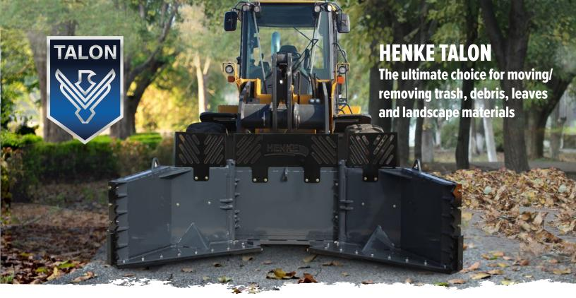
A GREAT ALTERNATIVE TO USING A GRAPPLE BUCKET, The Henke Talon is engineered to clear leaves, brush, debris, trash and landscape materials by hydraulically opening and closing the bucket claw to collect and compact material. The operator can easily maneuver to open and dump in the desired location. The Henke Talon works with most makes and models of Loaders.
