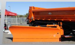
For enhanced operating capability, combine one of Henke's front plows (parallel or traditional lift) with postless or hydraulic wings.
