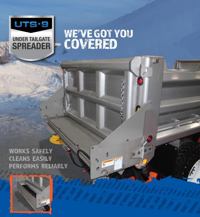
THE ONLY UNDER TAILGATE SPREADER with a FOLD FLAT COVER/BACKPLATE Easiest to clean. Easiest to maintain.
