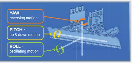
Rotates on 3 axes - reversing, up & down, oscillating to follow road contours
